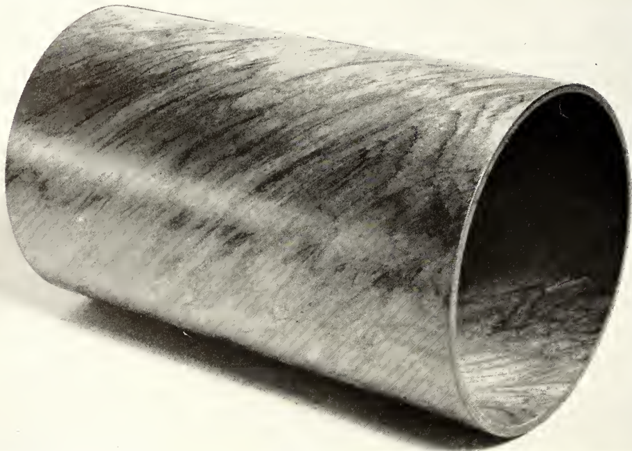
FIGURE 5-33.—Short section of tubular-molded plywood.
